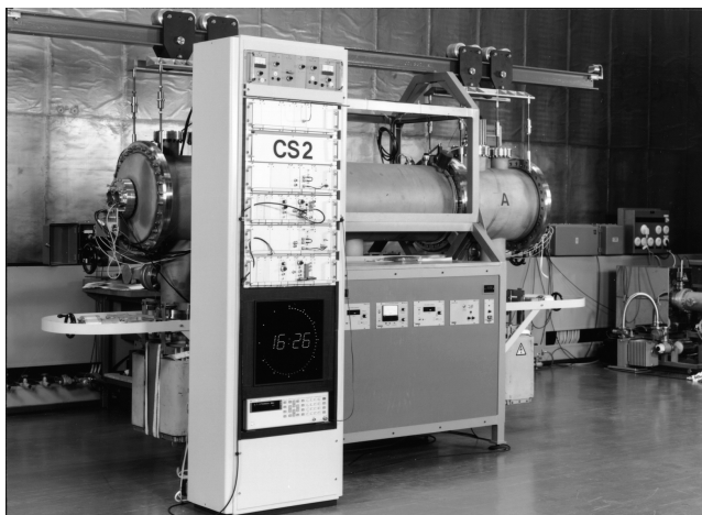
Figure 1: The cesium atomic clock C2 at the Federal Institute of Physics and Technology, Braunschweig (Brunswick), Germany.
